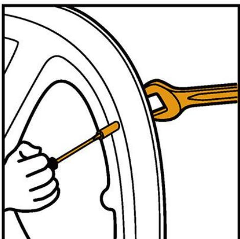
Tighten the valve by wrench and screw it ( Torque value must be  $\geq 4.5\text{Nm} \sim 5\text{Nm}$ )
